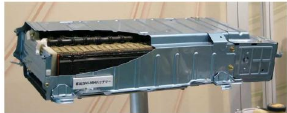
Exhibit 27. NiMH Car Battery For A Toyota Prius
